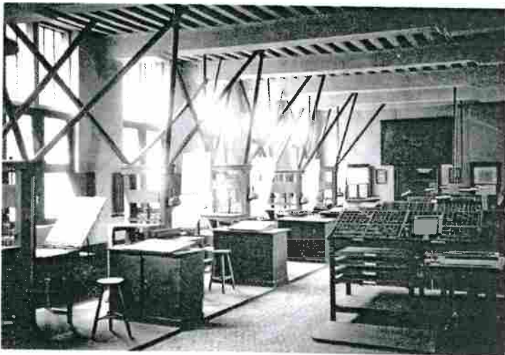
Left: A general view of part of the Plantin-Moretus Museum of Printing in Antwerp, once the press room of the Plantin publishing house. The heavy wooden presses on the left are fitted with struts from the ceiling. These steadied the presses as the continuous pulling action of the pressmen meant they were likely to move.
